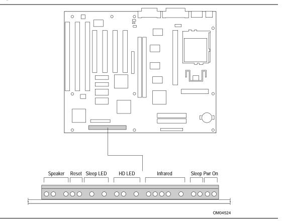
Figure 4. Front Panel I/O Connectors
